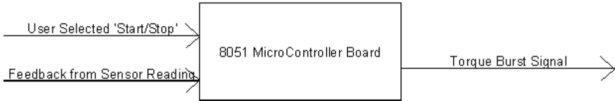
Figure 4. EMAC Microcontroller Development System Block Diagram
